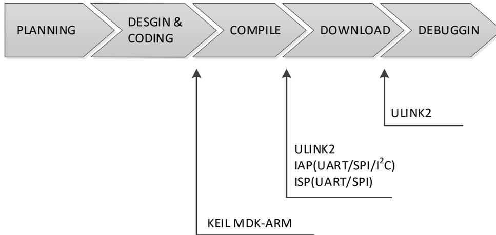
Figure 1 firmware development process
