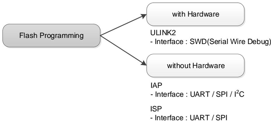
Figure 2 Methods to firmware programming
